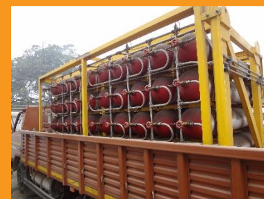
Cylinders with compressed biogas
